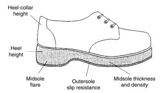
**Figure 1.** Features of shoe design that are thought to affect postural stability.
