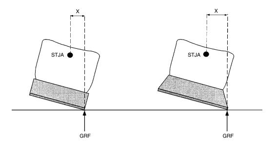
**Figure 4.** Effect of midsole flaring on foot pronation at heel strike during running. Ground-reactive force (GRF) is applied to the lateral plantar aspect of the shoe sole. The addition of a 30° lateral flare to a running shoe increases the lever arm for pronation (X) around the subtalar joint axis (STJA).
